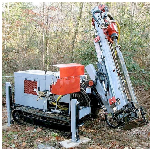
Figure 3. Blast-hole (bore-hole) drilling rigs are designed to be mobile and compact for working close to structures.
